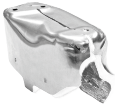
Direct shielding for oxidation catalytic converter
