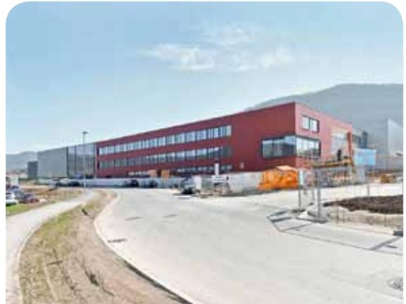
The new plastic housing module factory in Dettingen/Erms was designed to be as energy-efficient as possible. The production area covers nearly 20,000 m<sup>2</sup>. A 450 kW photovoltaic system was installed over approximately 3,000 m<sup>2</sup> of the roof space. Heat from the machinery and equipment is used to warm the factory space and offices, thus saving around 1,300 MWh of primary energy per year.
